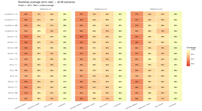
Fig. 7: Bootstrap coverage for error rate across all 48 scenarios and four methods. Green = 95% nominal. Red = undercoverage. The combined method is the only one that consistently reaches the target.
