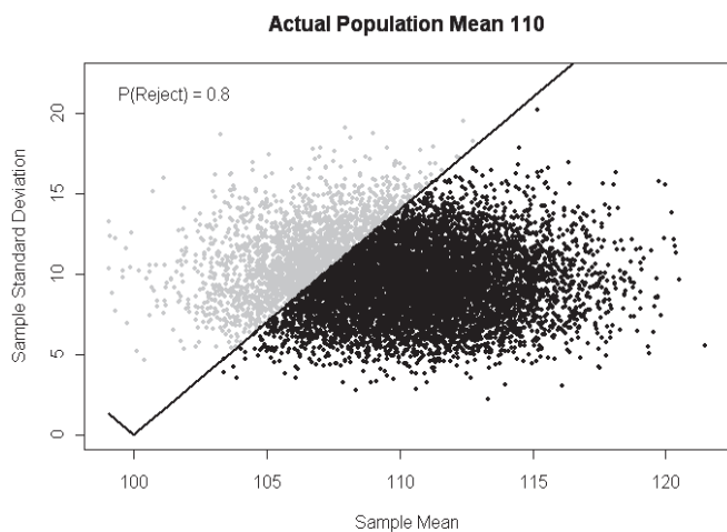
Figure 2. Sampling with a sample size of 10 from a normal distribution with \mu = 110 and \sigma = 10 and testing H_0: \mu = 100 against H_A: \mu \neq 100 when the null hypothesis is false, the dark dots show samples that reject H_0 and the pale dots show samples that do not reject H_0 .
