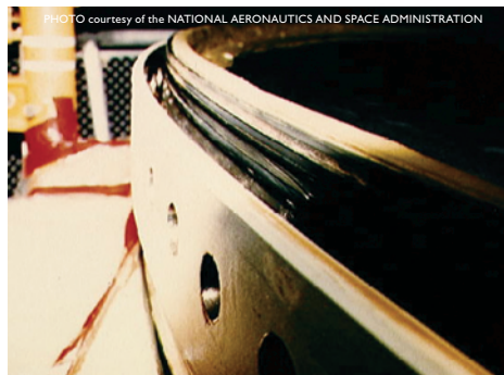
VIEW OF THE O-RING. This is a close-up photograph of the O-ring in the top of the aft segment of the right solid rocket booster (SRB) flown on Space Shuttle Mission 51-L. The photograph was released following a hearing on the space shuttle accident.
